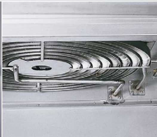
Kühlverdampfer cooling evaporator
